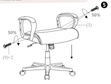
Note: Armrests are labeled with an "L" (left) or "R" (right) to show which sides they should be placed on.
