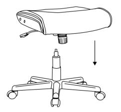
Position the assembled chair upright with the Seat Mechanism (4) facing down. Insert the Gas Lift (5) into the center hole of the Seat Mechanism (4) and press down until fully engaged.
