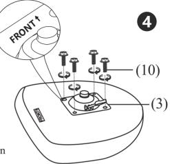
\*Be cautious as mis-threading the bolts will damage the seat.
