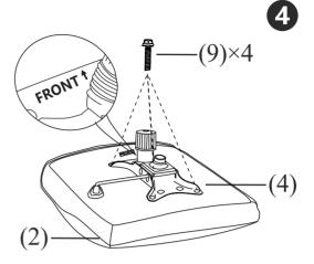
( Note! Don't make the direction wrong, make sure the front of the Mechanism **(4)** is facing the front of the Seat. )
