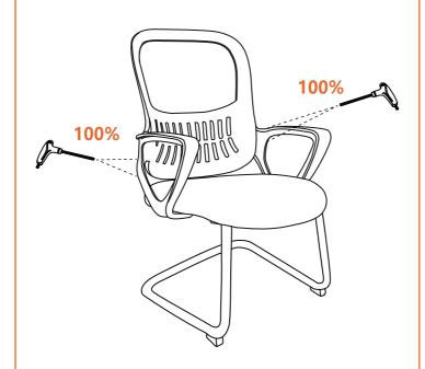
100% tighten the previously installed Bolts (E)\*4on the Armrests (C)\*1L\*1R.
