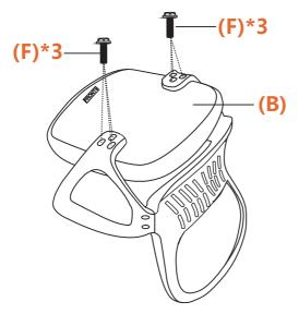
**NOTE:** The Seat is marked with "FRONT", please make sure the installation direction is correct.
