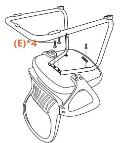
**NOTE:** As shown, make sure the Legs are facing correctly.
