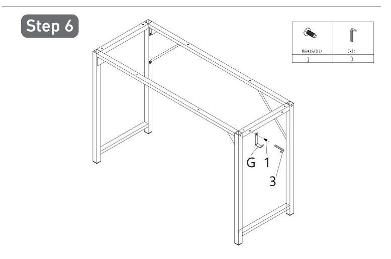
Attach Hook (G) to the Leg (D) with Screw (1)\*1.
