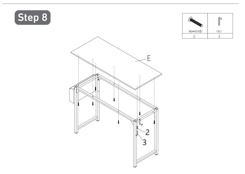
Attach Board (E) to the Legs (A&D) and Crossbars (B&C) with Screws (2)\*8.
