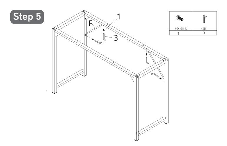
Attach Bar (F)\*2 to the Legs (A&D) and Crossbar (C) with Screws (1)\*4.
