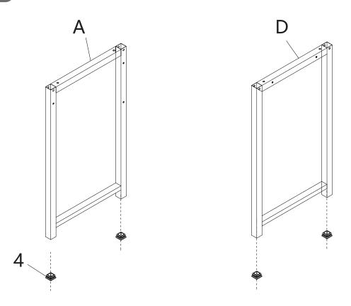
Attach Foot Pad (4)\*4 to the four feet of the Legs (A&D).
