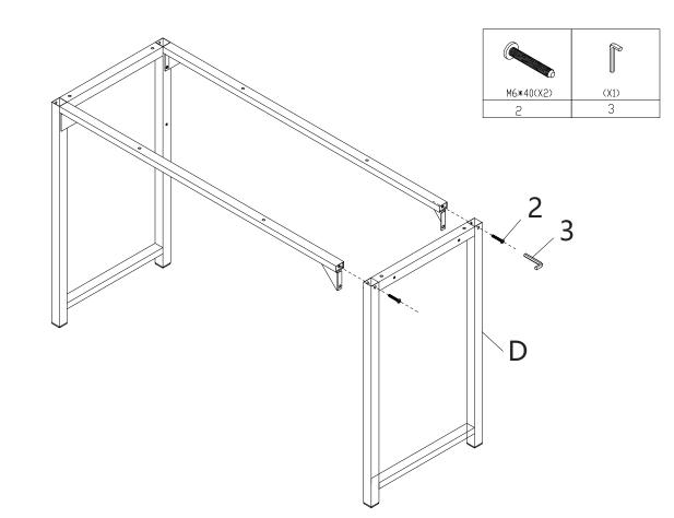
Attach Leg (D) to the installed Desk Frame with Screws (2)\*2. Please make sure the Legs are oriented correctly.
