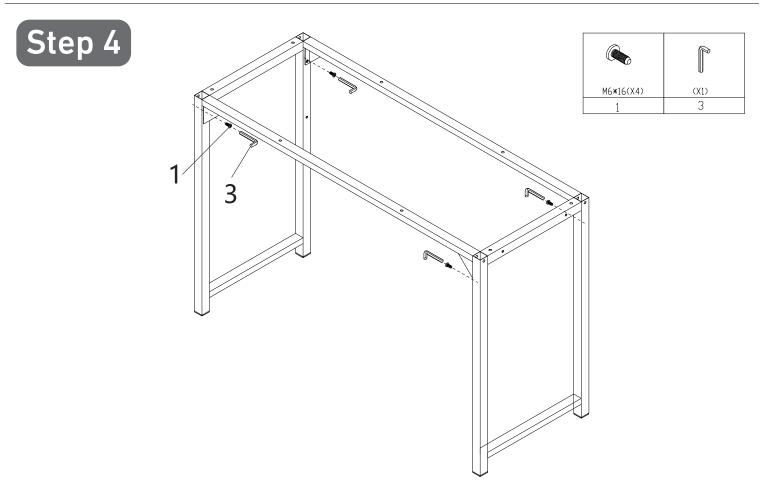
Secure the remaining four screw holes of the Crossbars (**B&C**) completely to the installed Desk Frame with Screws (1)\*4.
