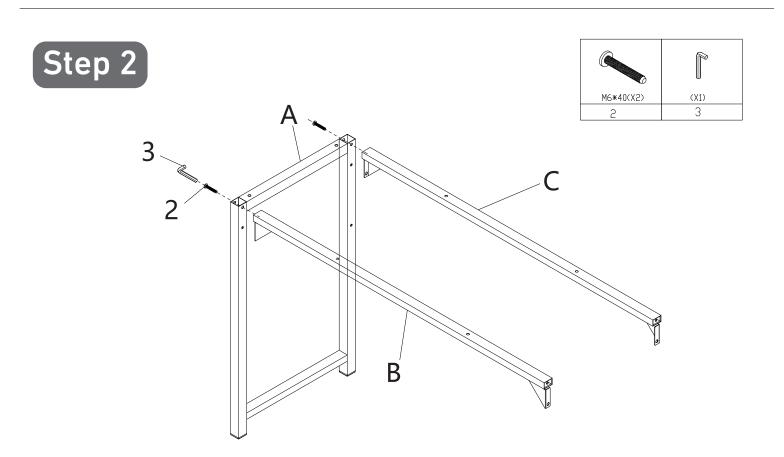
Attach Crossbar (B) to the **front** side of the Leg (A) and Crossbar (C) to its **back** side with Screws (2)\*2.
