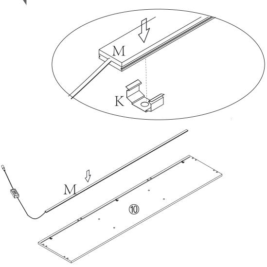
Note: The installation direction of the LED light strip can be left and right, either side is OK.
