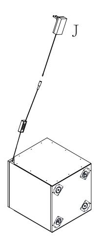
Note: The installation direction of the LED light strip can be left and right, either side is OK.
