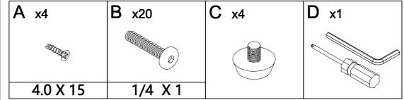
When the process of product assembly, please do not lock the screws at one time, but wait until all the screws are assembled to the position, and then straighten and flatten the product, and then tighten the screws of the same height in turn, so as to avoid unsmooth assembly and product tilt.
