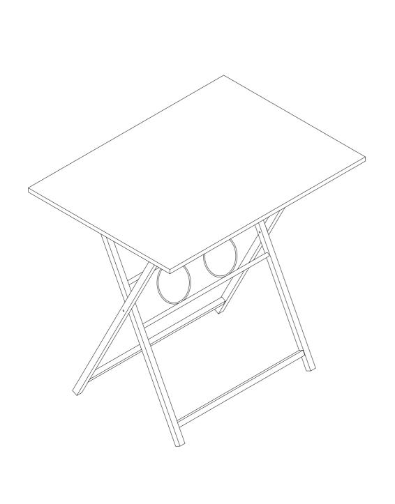
When the process of product assembly, please do not lock the screws at one time, but wait until all the screws are assembled to the position, and then straighten and flatten the product, and then tighten the screws of the same height in turn, so as to avoid unsmooth assembly and product tilt.
