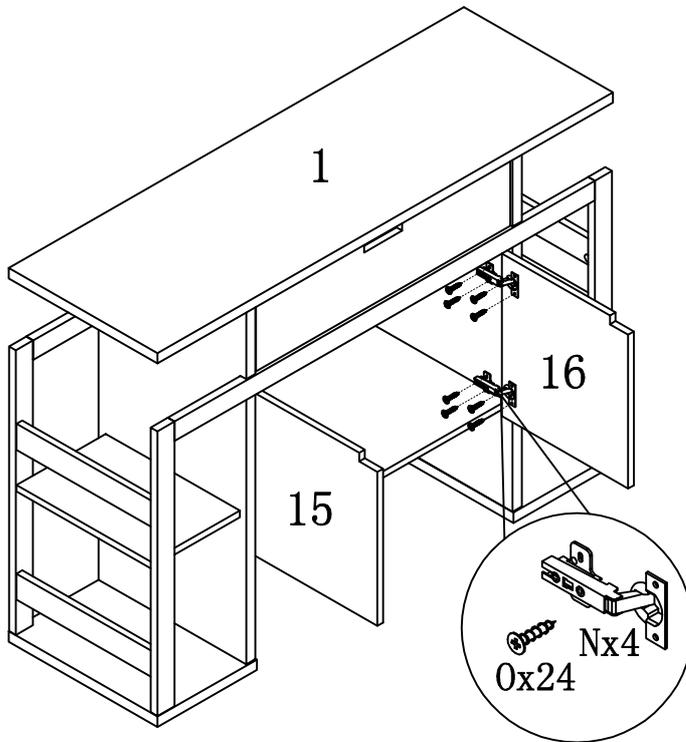
To adjust the door in or out, loosen this screw and push the door further in or push further out then retighten screws.
