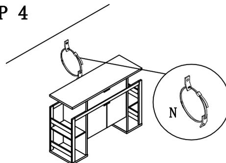
1. Insert strap thru bracket attached to wall, then thru bracket on item, and into head of strap.
