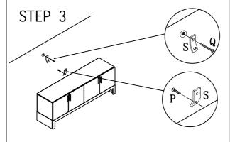
Insert drywall screw into metal bracket and into drywall anchor.
