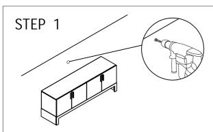
1. Find spot on wall 1" below top of item. 2. Using a drill bit slightly thinner than anchor, drill hole into drywall.
