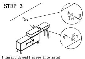
bracket and into drywall anchor.
