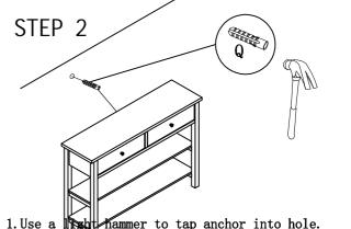
1. Use a hammer to tap anchor into hole.
