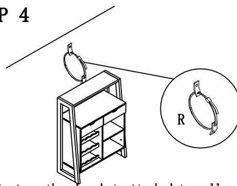
1. Insert strap thru bracket attached to wall, then thru bracket on item, and into head of strap.
