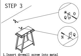
bracket and into drywall anchor.
