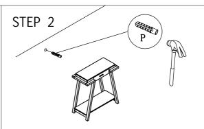
1. Use a light hammer to tap anchor into hole.
