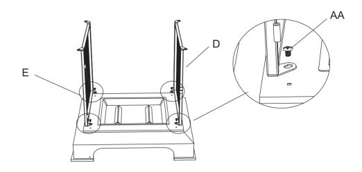
**Step 3:** Attached the Back Screen (C) with Side Panel (D) and (E) by using M6X10mm Bolts (AA). DO NOT tighten the bolts at this step.
