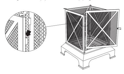
**Step 6**: Connect the Chimney (B) to the base by using M6X10mm Bolts(AA).
