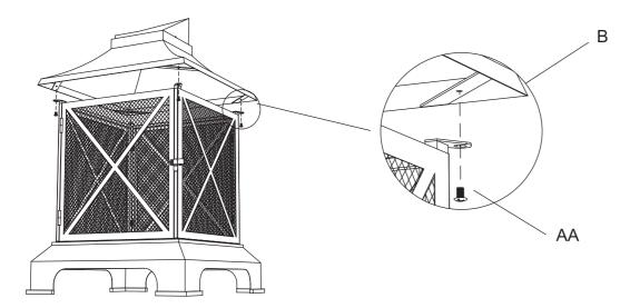
**Step 7**: Connect the Chimney Cover(A) to the Chimney Cover (B) by using M6X10mm Bolts(AA).
