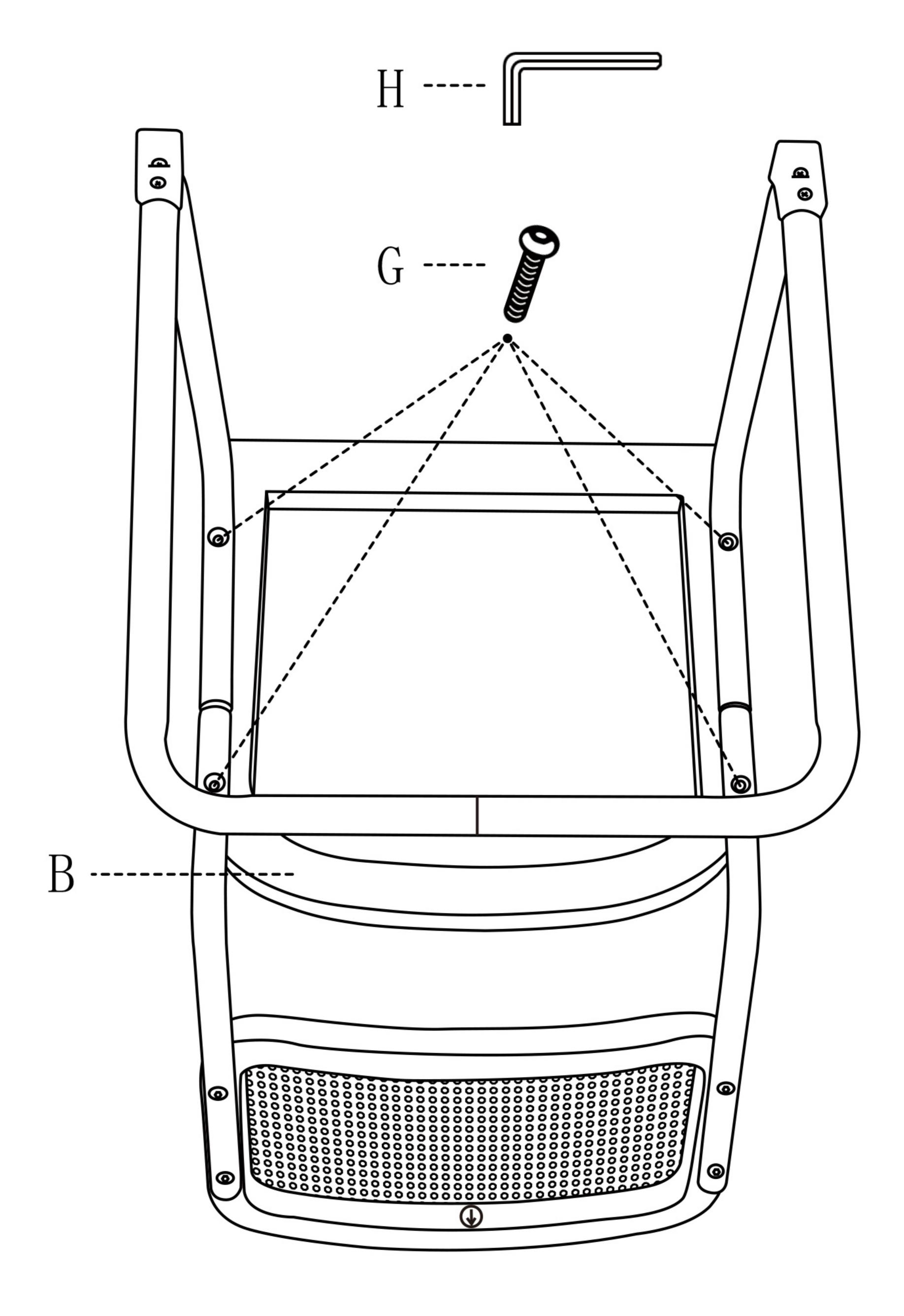
Insert Screws (G) by Wrench (H) for Part B, and tighten screws to 100%.
