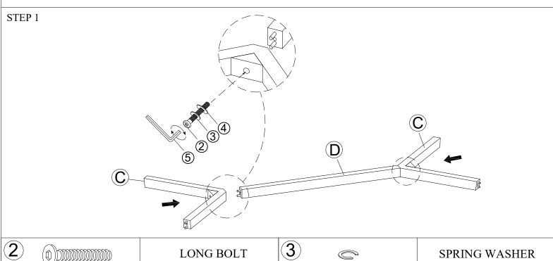
$(\emptyset)$ LONG BOLT SPRING WASHER (2PCS) (2PCS) Ø5/16"x13mm Ø5/16"x75mm **(5**) **4**) ALLEN KEY FLAT WASHER M4(2PCS) (1PC) Ø5/16"x19mm
