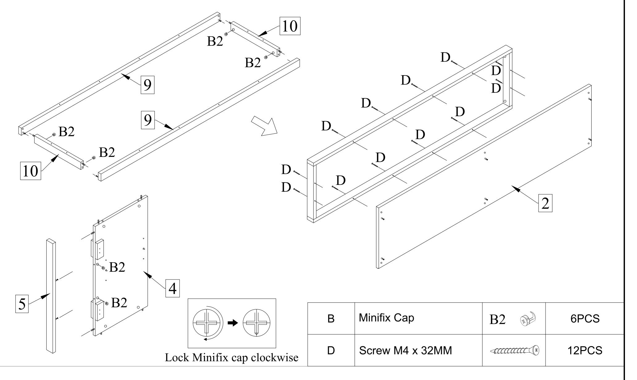
Step 3 : Connect Side & Center Panel (3,4,5) to Bottom Panel (2,9,10) and lock Minifix Cap (B2).
