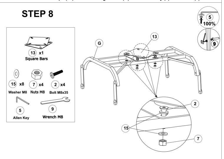
Connect Bars Square (14) & Rotating Frame (G) With Allen Key (5), Wrench (9).
