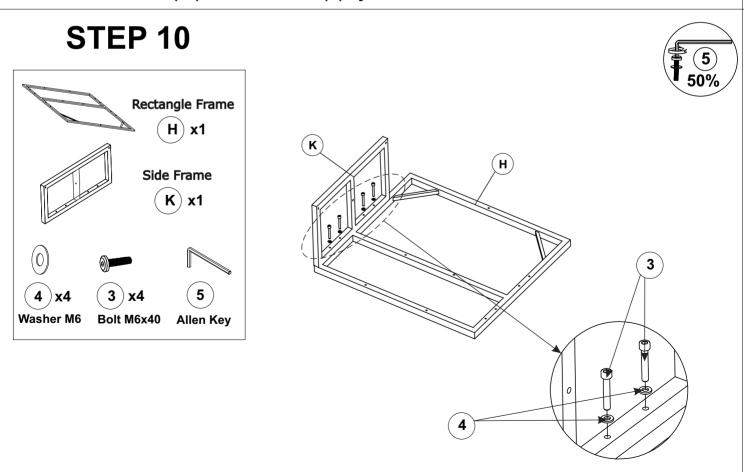
Connect Rectangle Frame (H) & Side Frame (K) With Allen Key (5).
