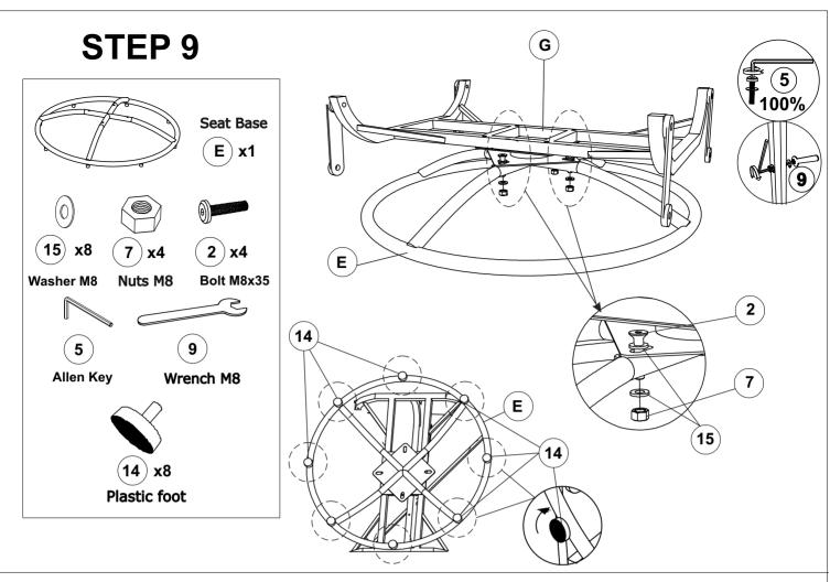
Connect Seat Base (E) & Rotating Frame (G) With Allen key (5) & Wrench (9). Connect Plastic foot (14) with Seat Base (E) by handle.
