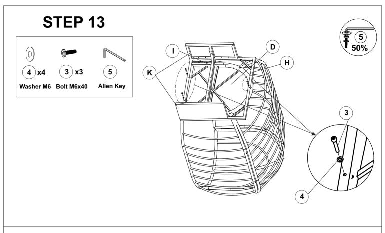
Connect Frame Of Step 12 & Frame Of Step 6 With Allen Key (5).
