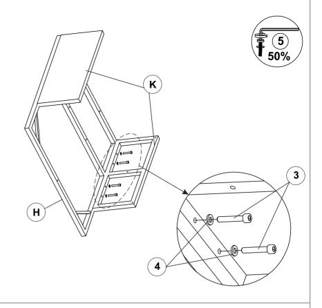
Connect Rectangle Frame (H) & Side Frame (K) With Allen Key (5).
