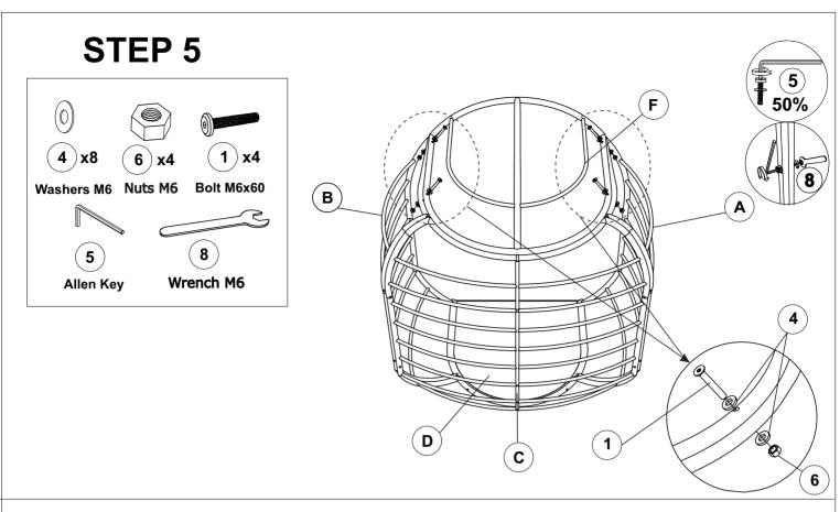
Connect Seat Cover (F) & Right Arm (A), Left Arm(B) With Allen Key (5) & Wrench (8).
