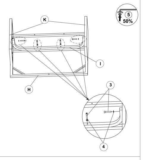
Connect U-Shape Frame (I) & Side Frame (K), Rectangle Frame (H) With Allen Key (5).
