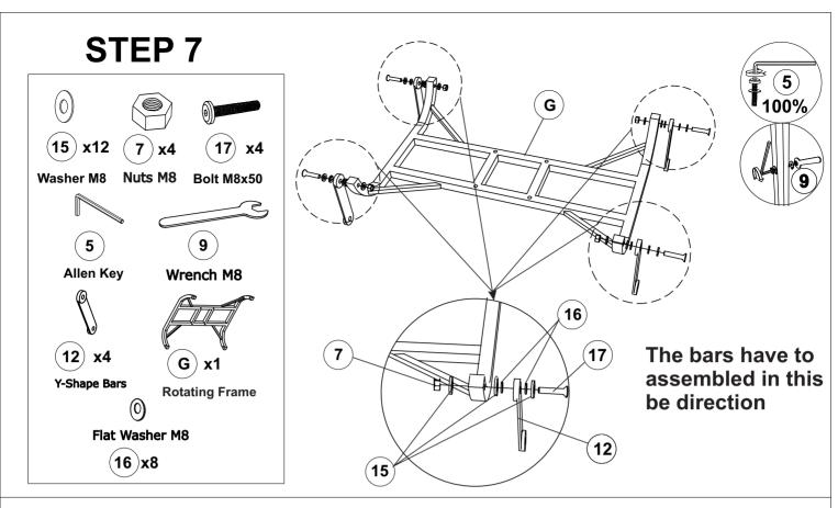
Connect All Bars Y-Shape (13) onto Rotating Frame (G) With Allen key (5) & Wrench (9).
