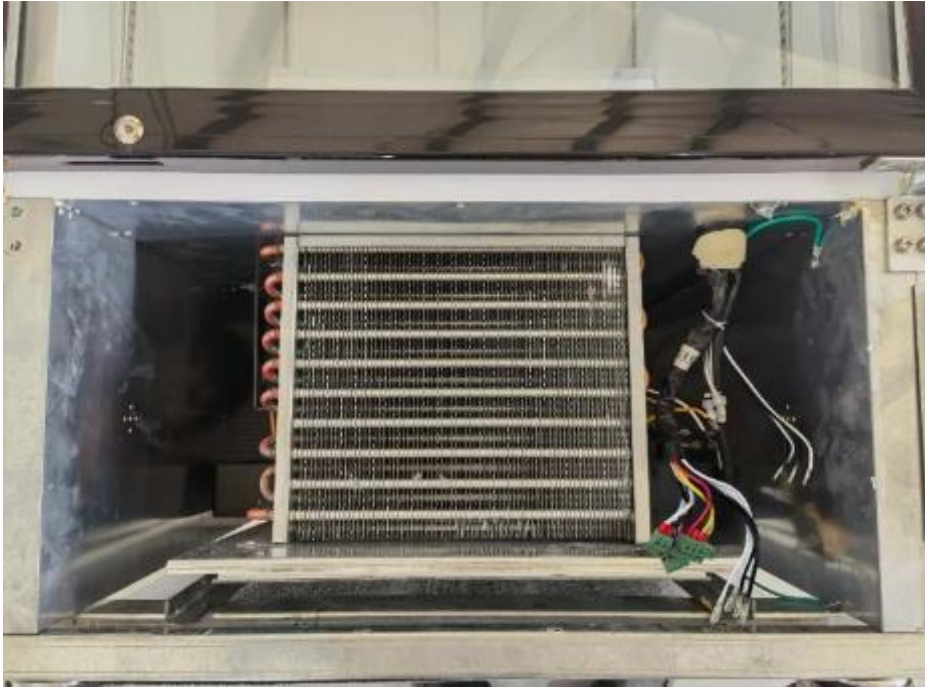
Photo 39a - Condenser part view - ST27BFGC
