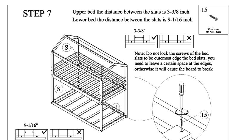
Note: Do not lock the screws of the bed slats to be outemost edge the bed slats, you need to leave a certain space at the edges, ortherwise it will cause the board to break
