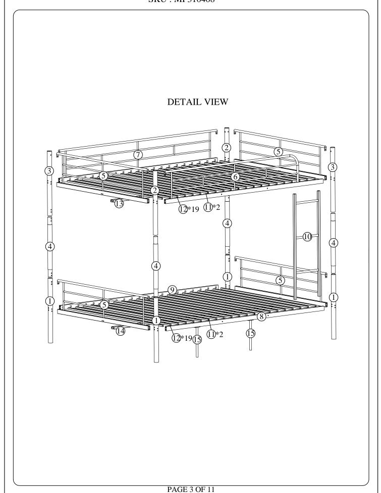
**PART LIST** (15) x2 (5) x4 (1) x4 (2) x2 (3) x2 6x10 0 (7) x1 8x10 0 9x1(1) x4 (12) x38 0 x1 (13) x1 (14) x1 HARDWARE LIST End cap **G**Connect End cap (F) Allen key Hex nut (A) Bolts Bolts © Bolts wall **(6)** 1/4\*40 1/4 Ø42 4\*59 1/4\*60 1/4\*40 Ø19 1/4\*15 16PCS 2PCS 1PC 2 SET 4PCS 36PCS 8PCS 35PCS
