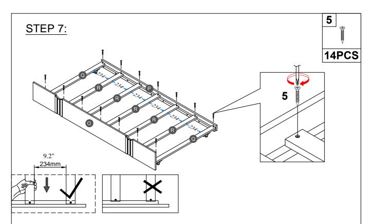
Note: Do not lock the screws of the bed slats to the outermost edge of the bed slats, you need to leave a certain space at the edges, otherwise it will cause the board to break.
