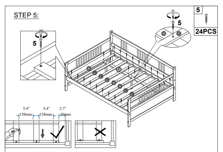
Note: Do not lock the screws of the bed slats to the outermost edge of the bed slats, you need to leave a certain space at the edges, otherwise it will cause the board to break. Do not lock the bed slats on the edge of the wood, please hold firmly before screwing, hold it in place with one hand, then lock the screw.
