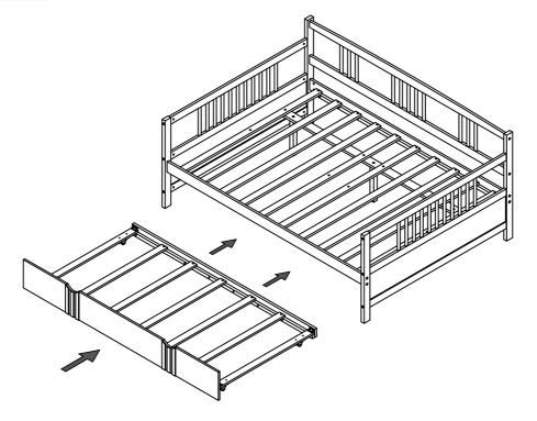
Push Trundle under the bottom of Bunkbed.
