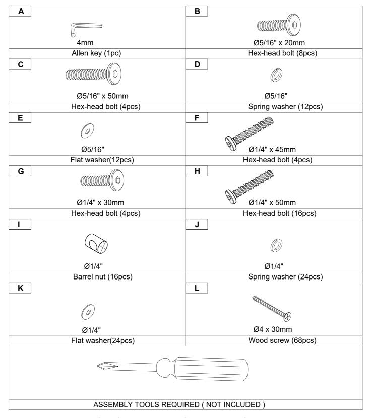
Read this instruction carefully. See hardware and furniture part list for guidance. Be sure all parts are complete, before you assemble. Place all wooden furniture parts on a clean and flat soft surface to prevent from being scratched. Follow the figure to start assembling.
