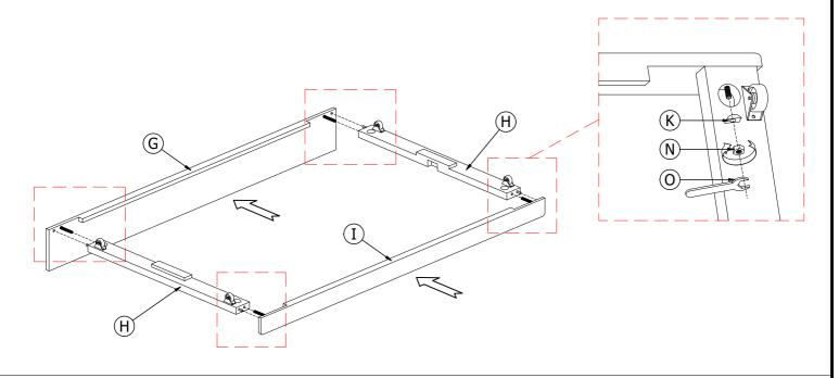
Step 6. Place put the Trundle support slat(J) with mount wheels the into the Trundle side(H). Then, put the Slat roll(F) and arrange it neatly. Finally, all togethertighten they are by Screws(Q) as guide.
