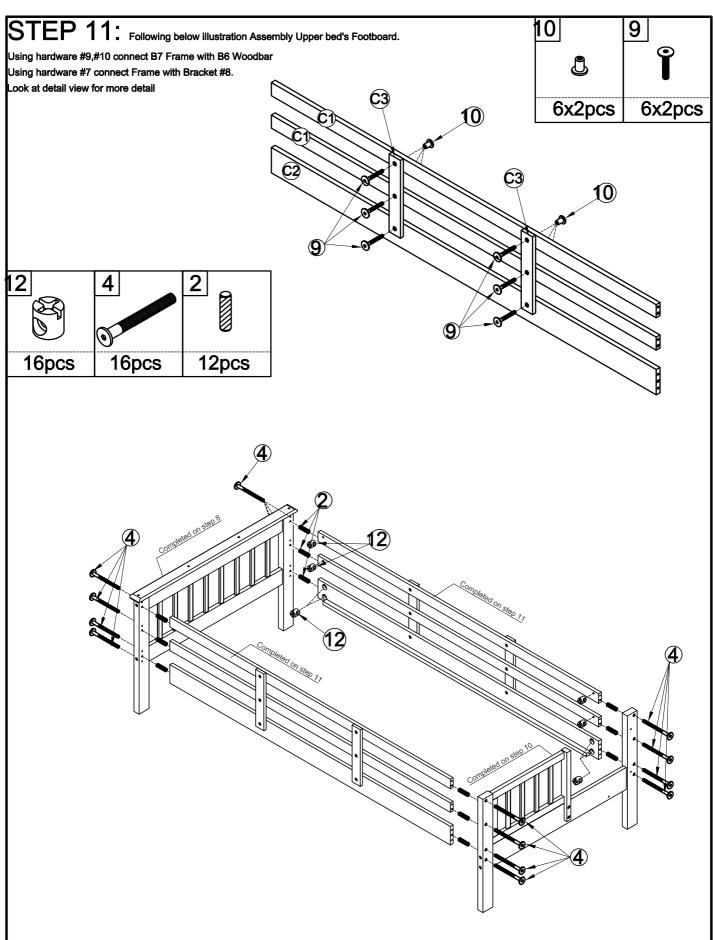
STEP 12: Following below illustration Using hardward #4,#12 and dowel #2
