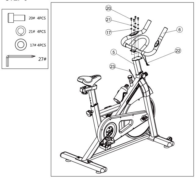
The Handle Frame (6) is fixed on the Handle Post (5) with Flat washers (17), the Spring washers (21) and the Button head bolts (20), and tightened with an inner hexagonal wrench (27).
