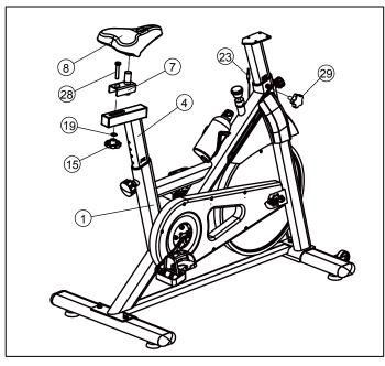
The Saddle Adjustment Frame (7) is installed in the Saddle Post (4) and fixed with the Flat washer (19), an six angle bolts (28) and a adjusting nut (15). Then the Saddle (8) is arranged on the Saddle Adjustment Frame (7), and is fixed and tightened with the open wrench (25). Install adjusting nut(29) on main body(1).
