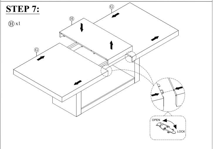
Open the 4 lockers under the Top Panel (G), drag them to side, put the Medium Panel (H) into the middle, fit the posotion then close the lockers.
