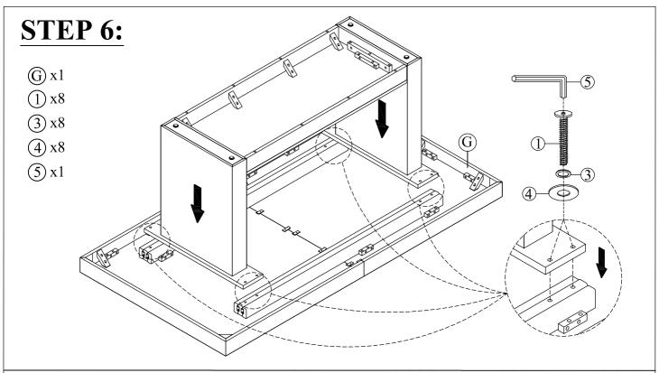
Connect the Part from Step 2 and Top Panel (G), tighten Bolt (1), Flat Washer (3), Lock Washer (4) with Allen Key (5)
