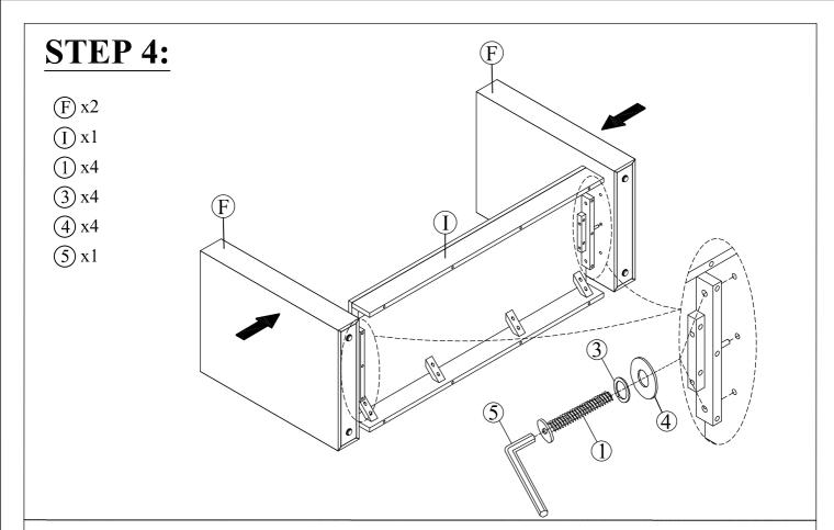
Connect the Leg (F) and Table base center (I), tighten Bolt (1), Flat Washer (3), Lock Washer (4) with Allen Key (5)
