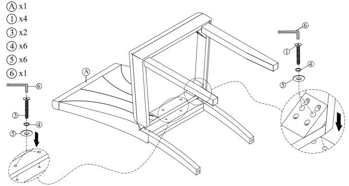
Connect the Part from Step 1 and Chair Back (A), tighten Bolt (1), Bolt (3), Flat Washer (4), Lock Washer (5) with Allen Key (6)
