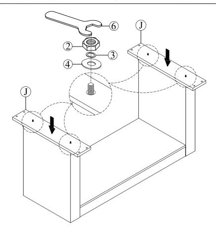
Connect the Part from Step 1 and Panel (J), tighten Hex nut (2), Flat Washer (3), Lock Washer (4) Wrench (6)
