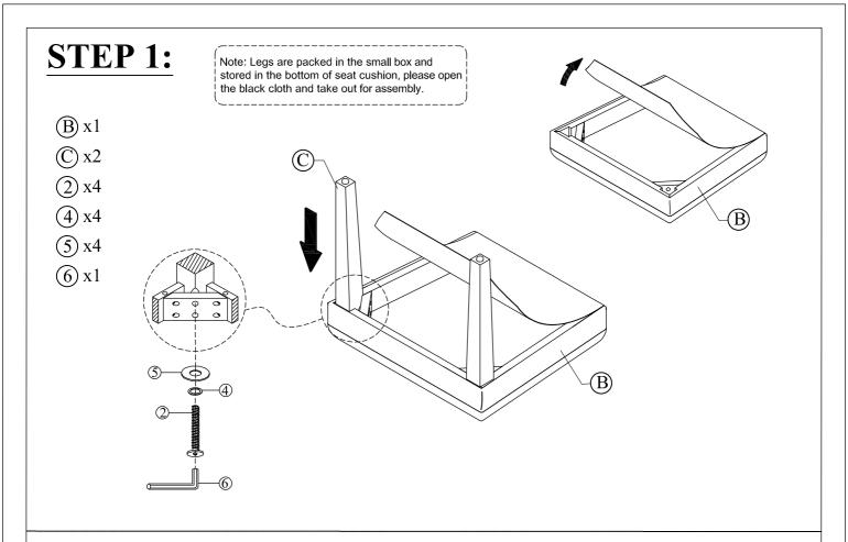
Connect the Front Leg (C) and Cushion seat (B), tighten Bolt (2), Flat Washer (4), Lock Washer (5) with Allen Key (6)
