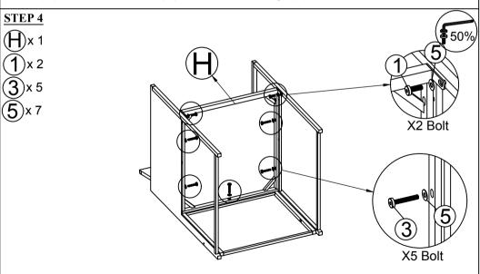
Connect The Part from STEP 3 & Seat Chair (H), tighten Bolt (1),(3), Flat Washer (5) with Allen Key (7).
