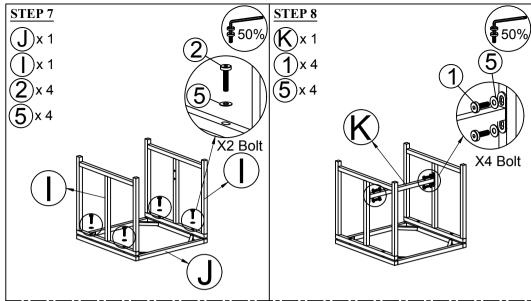
Connect The Seat Stool (J) & Leg Stool (I), tighten Bolt (2), Flat Washer (5) with Allen Key (7) Connect The Part from STEP 7 & Support Stool (K), tighten Bolt (1), Flat Washer (5) with Allen Key (7).
