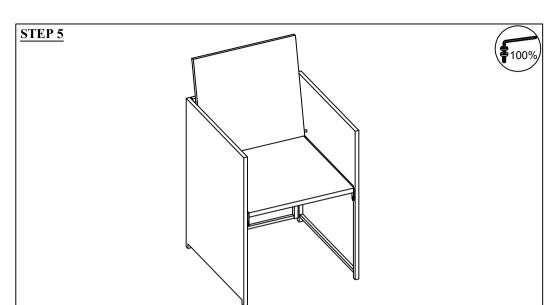
Put the Chair upright and make sure all legs are level, then firmly tighten Bolts with Allen Key (7)
