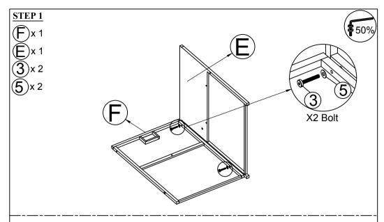
Connect The Arm Right Chair (E) & Behind Chair (F), tighten Bolt (3), Flat Washer (5) with Allen Key (7).
