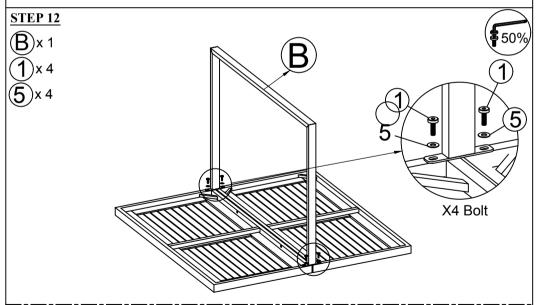
Connect The Part from STEP 11 & Leg Table (B), tighten Bolt (1), Flat Washer (5) with Allen Key (7).
