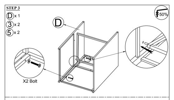
Connect The Part from STEP 2 & Arm Right Chair (D), tighten Bolt (3), Flat Washer (5) with Allen Key (7).
