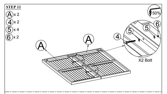
Connect The two Top Table (A), tighten Bolt (5), Flat Washer (5), Nut (6) with Allen Key (7), Key (8).
