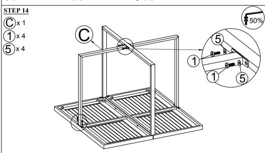
Connect The Part from STEP 13 & Side Leg Table (C), tighten Bolt (1), Flat Washer (5) with Allen Key (7).
