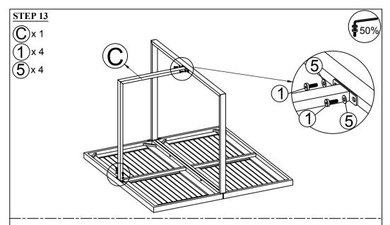
Connect The Part from Step 12 & Side leg Table (C), tighten Bolt (1), Flat Washer (5) with Allen Key (7).
