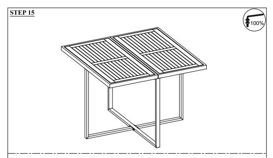
Put the Table upright and make sure all legs are level, then firmly tighten Bolts with Allen Key (7)
