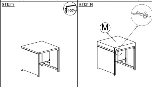
Put the Stool upright and make sure all legs are level, then firmly tighten Bolts with Allen Key (7)
