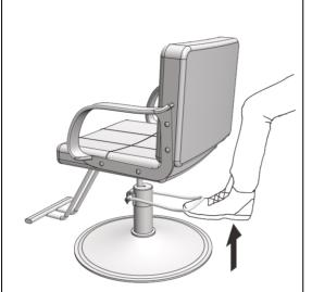
**Lock**: Lift the foot pump rod upward, and the rotation and lifting functions are locked.
