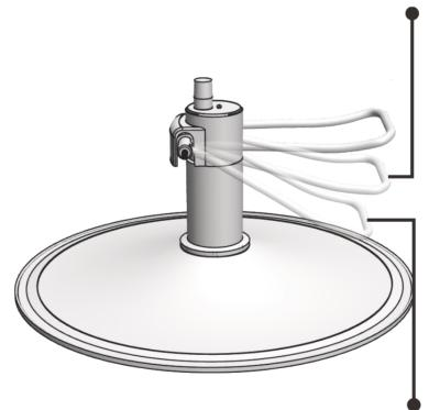
**Seat down:** Downhill the foot pump rod and hold still to lower the seat.
