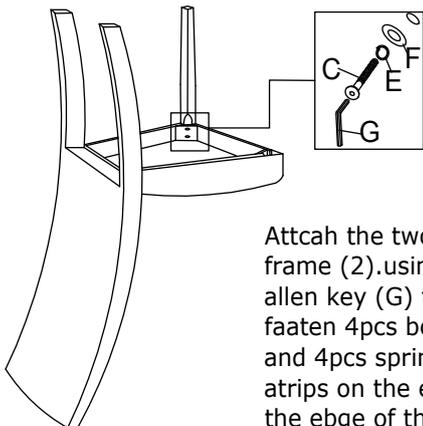
Attach the two front leg(3) to the seat frame (2). using the allen key (G) to fully fasten 4pcs bolt(C). 4pcs flat washer (E) and 4pcs spring washer(F). stick velcro strips on the edge of non woven to it on the edge of the seat frame.
