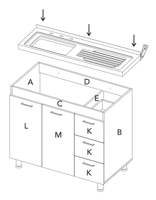
\*Apply a thick bead of silicone to all edges of the counter to seal and provide protection.
