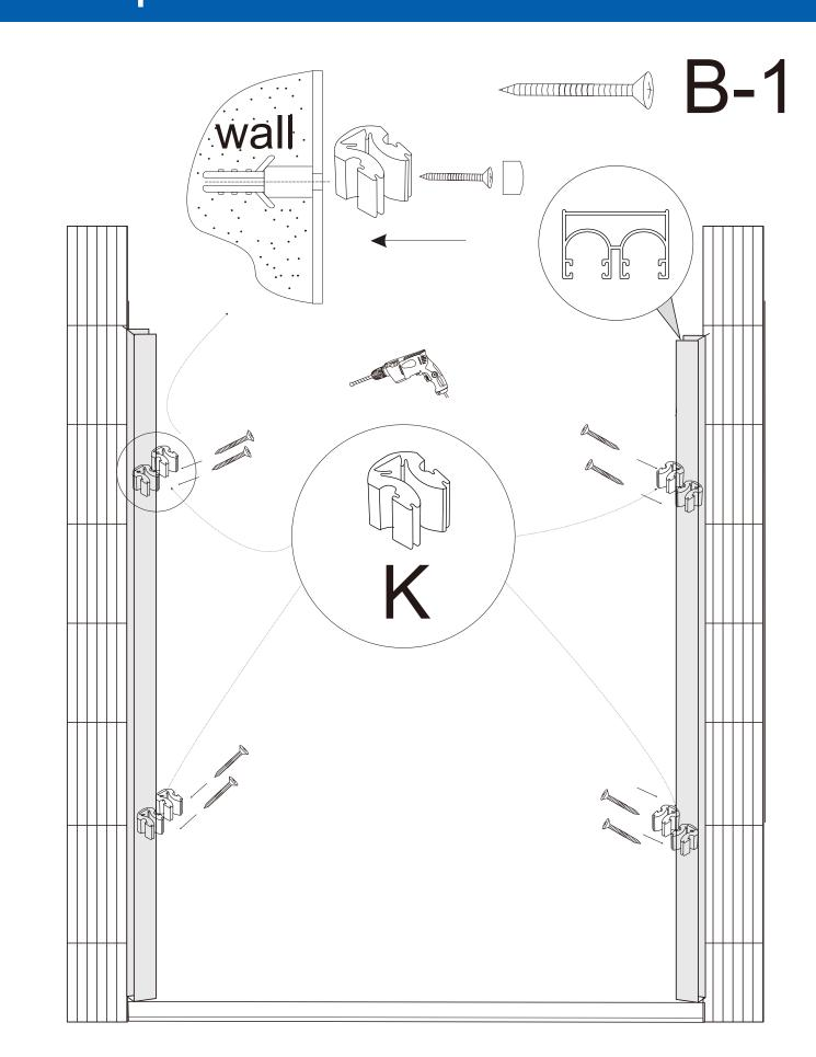
Change a cross bit on electric drill, Match holes on K with holes on wall, Use A-1 to fix (1\*B-1 for each hole)
