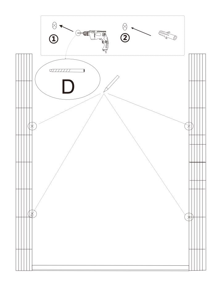
Mark 4 holes for fixing vertical frames, Match D on electric drill to punch 8 holes, Insert 8 expansion bolts
