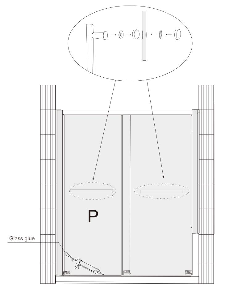
Make sure both sides are with rubber piece between glass and handle
