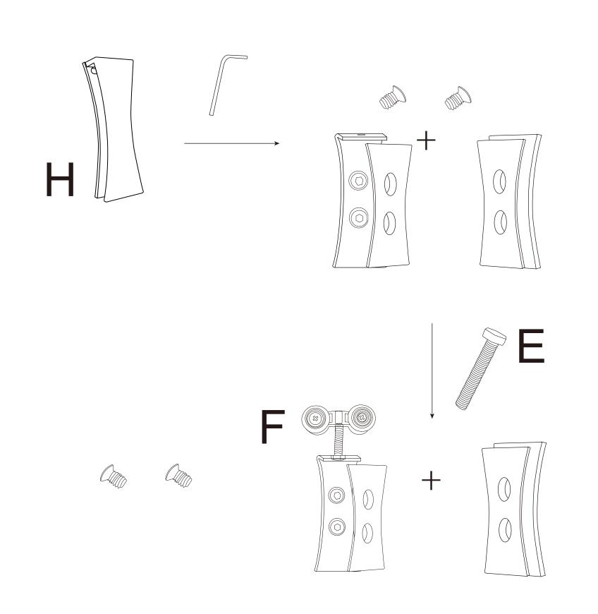
Here are 2 paths on up track, put 2 roller sets in each path, do not lock these 2 screws at the end of this step
