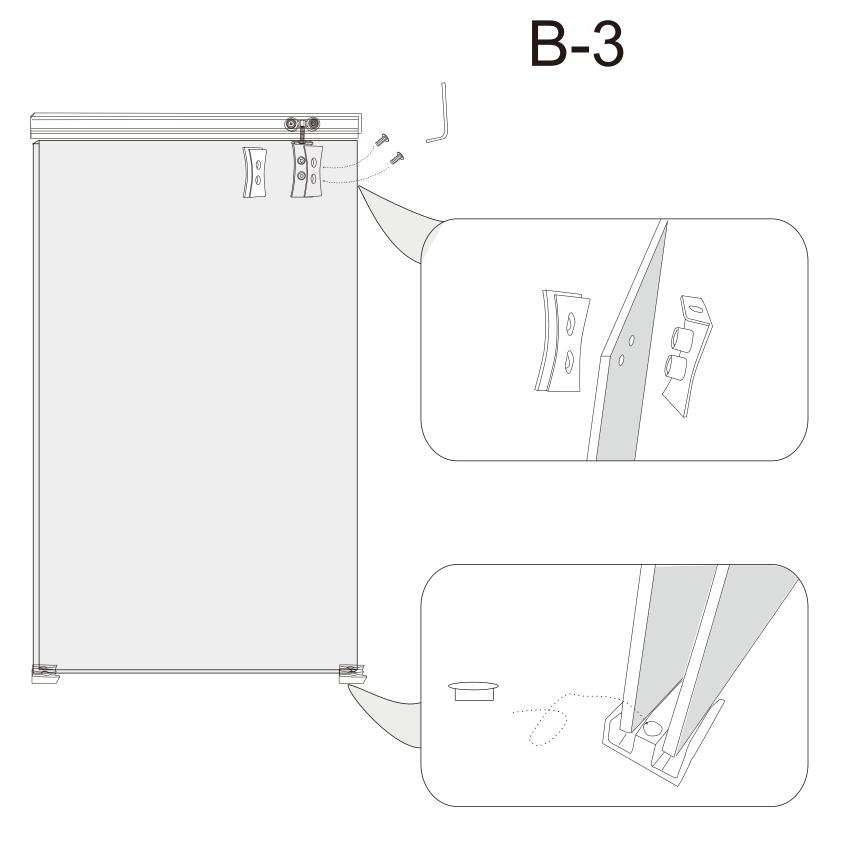
Ask someone to lift the glass for fixing it with hinges on rollers, leave a little space between glass and H
