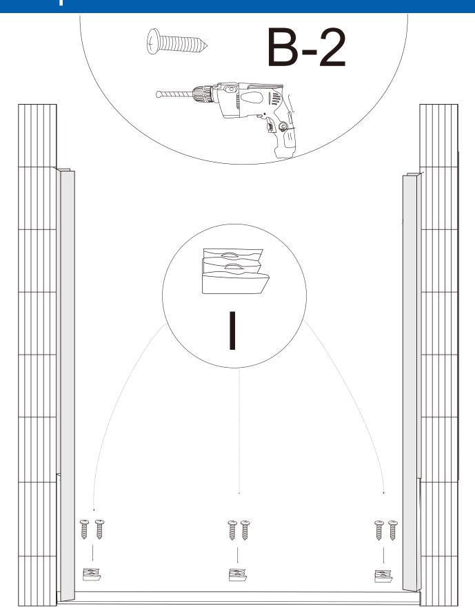
Put 3\*I on exact places shown on picture Use A-2 to fix (there are no holes on down track, 2\*B-2 for each I)
