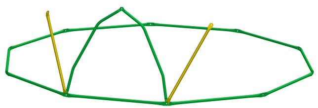
Repeat the same step to attach a Yellow Tube(2#) and a Green Tube(1#) to the next joint, and secure with 1pc 8 x 30mm Bolt(7#), 1 pc M8 Washer(8#) and 1pc M8 Nut(9#).
