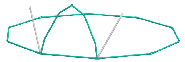
Repeat the same step to attach a Silver Tube(2#) and a Green Tube(1#) to the next joint, and secure with 1pc 8 x 30mm Bolt(7#), 1 pc M8 Washer(8#) and 1pc M8 Nut(9#).
