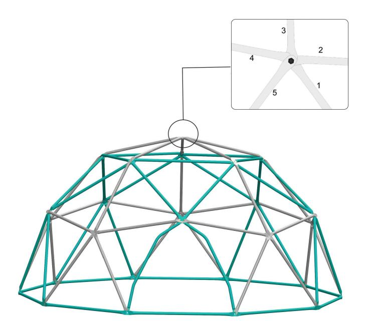
Install the Climbing Grips to cover the bolt on each of the joint. Small Climbing Grips (10 pcs) should be installed on the bottom joints. Large Climbing Grips (16 pcs) should be installed on the joints not touching the ground.
