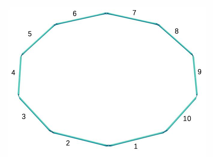
Slide an M8 Washer(8#) over M8 x 30mm Bolt(7#), then slide the Bolt(7#) through the joint of 2pcs Green Tubes(1#) on the ground, 1pc Silver Tube(2#) and 1pc Green Gate Tube(4#) in the order indicated by the numbers. Secure Bolt(#7) with an M8 Nut(#9).
