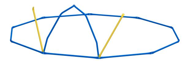
Repeat the same step to attach a Yellow Tube(2#) and a Blue Tube(1#) to the next joint, and secure with 1pc 8 x 30mm Bolt(7#), 1 pc M8 Washer(8#) and 1pc M8 Nut(9#).
