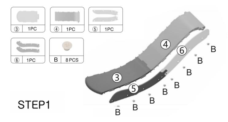
Connect Part 3, 4, 5, 6 together as shown, and secure with 8pcs Screw B.
