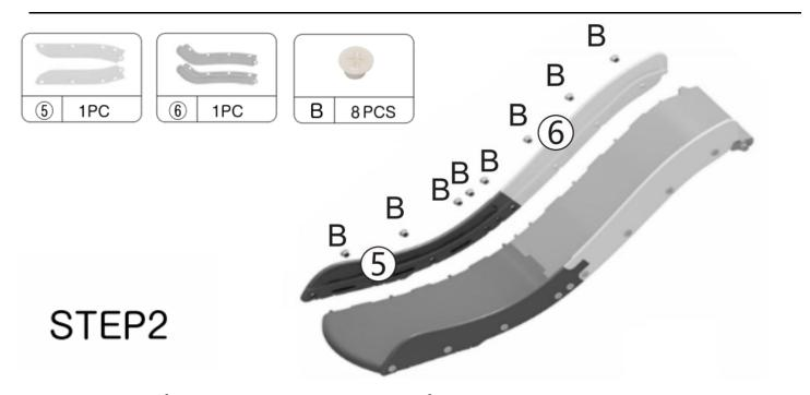
Connect the Part ⑤ to Part ⑥. Then attach the assembled parts to the STEP 1 assembled parts, secure with 8 Screw B
