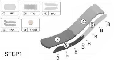
Connect Part ③, ④, ⑤, ⑥ together as shown, and secure with 8pcs Screw B.
