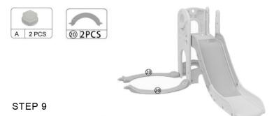
Connect the 2 Part 20 to the STEP 8 assembled parts, Secure with 2 Screw A
