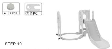
Connect the Part  ${\mathfrak T}$  to the STEP 9 assembled parts, secure with 2 Screw A.
