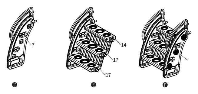
Insert the 2pcs 17 and 1pc 14 into the holes in the Part 7, and secure with 3pcs Screw 26 each side.
