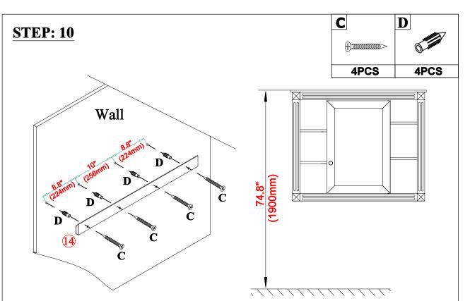
Draw the spacing between the walls and the No.14, punch holes in the wall, and fix the No.14 to the wall with screws.
