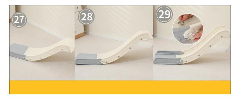
Connect the Part #17 to the completed part in STEP 26 and secure with Screw #29 and Screw #36.
