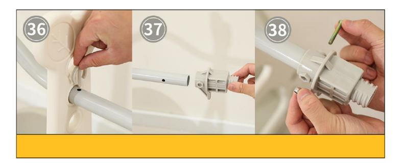
Insert the Lock Pin #34 into the holes of the Part #23 to secure the swing.
