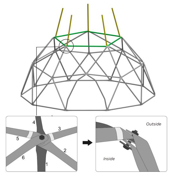
Slide Yellow Tube(#Q) into Yellow Tube(#P), secure the joint on top with 1pc M8 x 40mm Bolt(#E), 1pc M8 Washer(H) and 1pc M8 Nut(#K).
