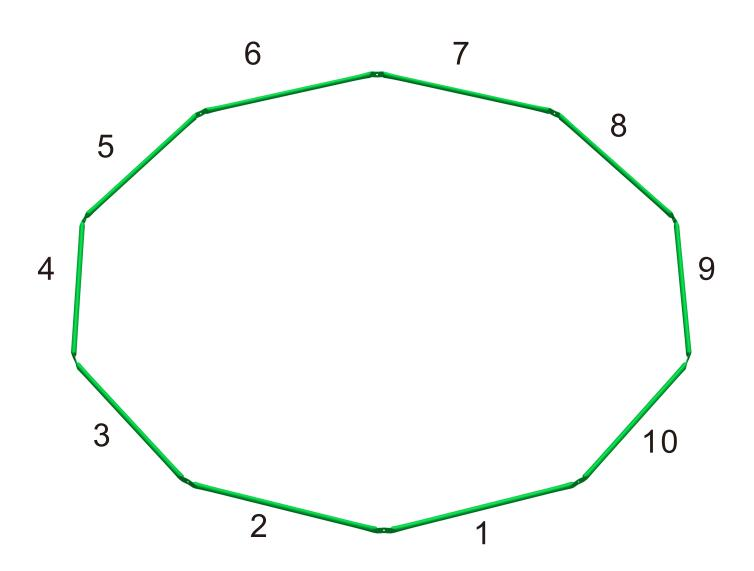
Slide an M8 Washer(#H) over  $\phi 10 \times 25$ mm Bolt(#F), then slide the Bolt(#F) through the joint of 2pcs Green Tubes(#A) on the ground, 1pc Yellow Tube(#B) and 1pc Green Left Gate Tube(#N) in the order indicated by the numbers. Slide another M8 Washer(#H) over the Bolt(#F) and secure with an M8 Nylon Nut(#G).
