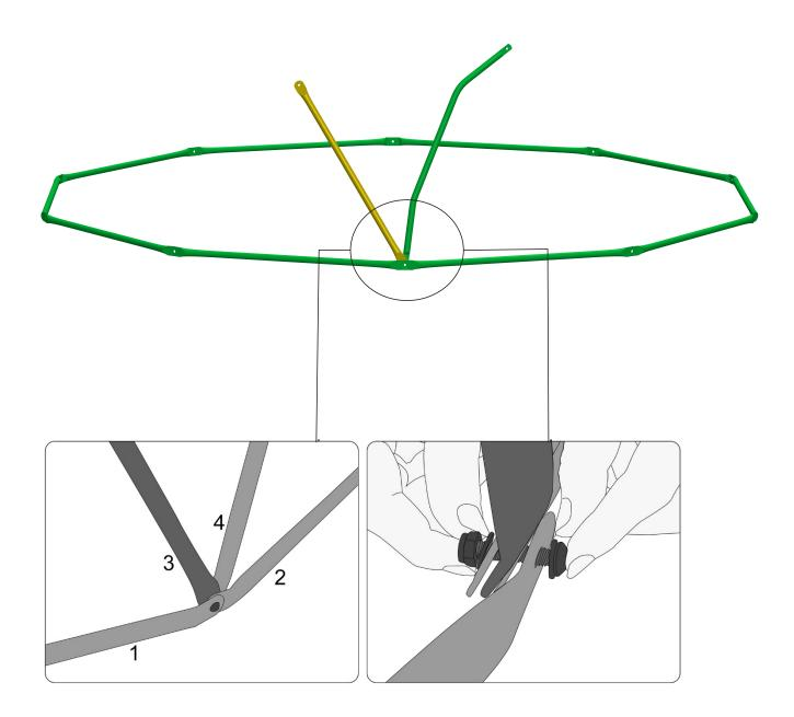
Attach a Yellow Tube(#B) and the Green Right Gate Tube(#O) to the bottom joint in the right, slide a  $\phi 10 \times 25$ mm Bolt(#F) through an M8 Washer(#H), the four tubes (in the same order indicated above), another M8 Washer(#H) and an M8 Nylon Nut(#G).
