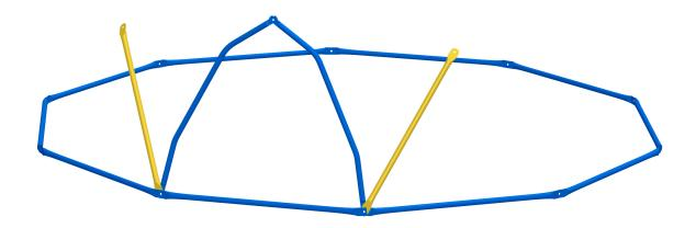
Repeat the same step to attach a Yellow Tube(#2) and a Blue Tube(#1) to the next joint, and secure with 1pc M8 x 30mm Bolt(#7), 1 pc M8 Washer(#8) and 1pc M8 Nut(#9).
