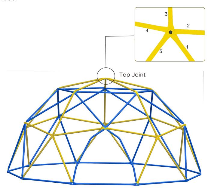
Install the Climbing Rock to cover the bolt on each of the joint. Small Climbing Rocks (10 pcs) should be installed on the bottom joints. Large Climbing Rocks (16 pcs) should be installed on the joints not touching the ground.
