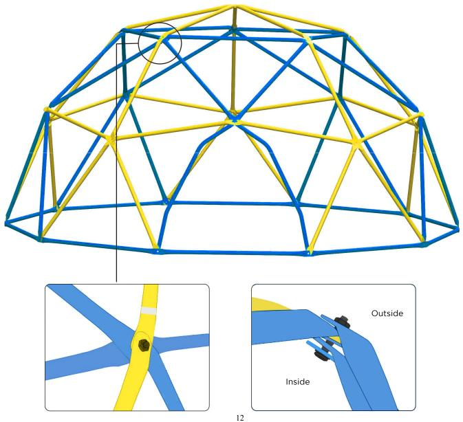
Secure the joint on top with 1pc M8 x 30mm Bolt(#7), 1pc M8 Washer(#8) and 1pc M8 Nut(#9).
