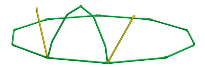
Repeat the same step to attach a Yellow Tube(#B) and a Green Tube(#A) to the next joint, and secure with 1pc  $\phi$ 10 x 25mm Bolt(#F), 2 pcs M8 Washer(#H) and 1pc M8 Nylon Nut(#G).
