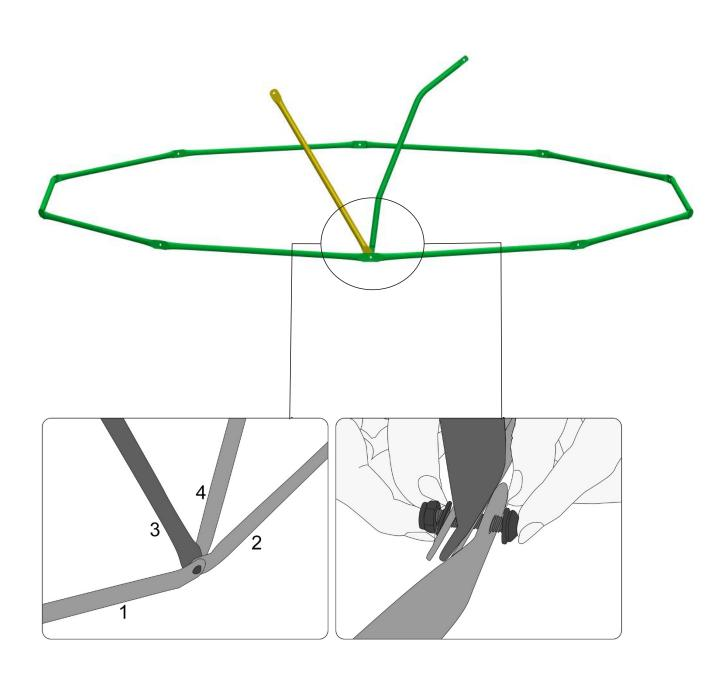
Attach a Yellow Tube(#B) and the Green Right Gate Tube(#O) to the bottom joint in the right, slide a  $\phi$ 10 x 25mm Bolt(#F) through an M8 Washer(#H), the four tubes (in the same order indicated above), another M8 Washer(#H) and an M8 Nylon Nut(#G).
