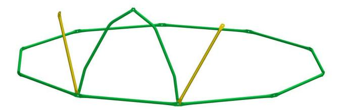
Repeat the same step to attach a Yellow Tube(#B) and a Green Tube(#A) to the next joint, and secure with 1pc  $\phi$ 10 x 25mm Bolt(#F), 2 pcs M8 Washer(#H) and 1pc M8 Nylon Nut(#G).
