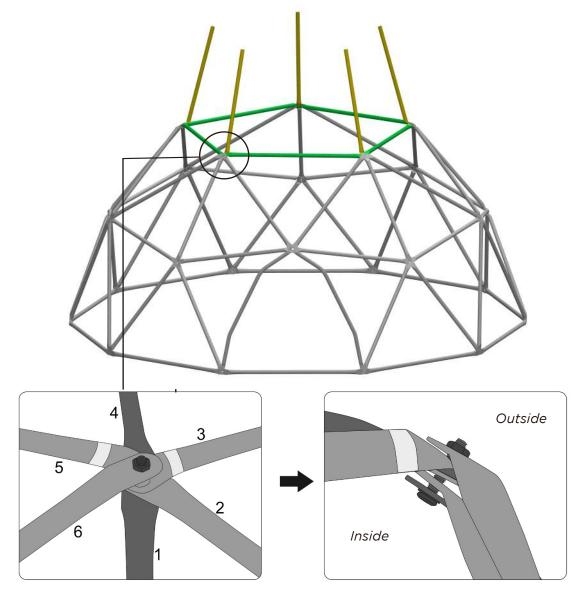
Slide Yellow Tube(#Q) into Yellow Tube(#P), secure the joint on top with 1pc M8 x 40mm Bolt(#E), 1pc M8 Washer(H) and 1pc M8 Nut(#K).
