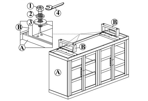
Step 2: Turn the Server to upright position. (\**Note: It is recommended to use two or more people to turn the Server*). Place the Server on flat surface and adjust the Leveler under the Metal Legs (B) until level and does not wobble.
