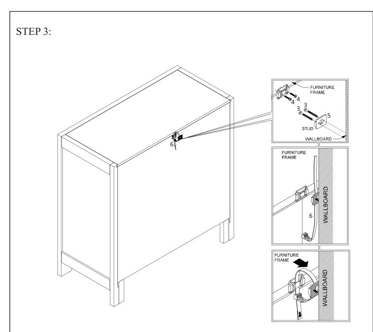
**STEP (A)** Locate a wall stud behind your furniture. Position a bracket on the stud approximately 1'' below the top of the furniture. Mark & drill pilot hole into the center of the stud with a 3/32" drill bit. Attach the bracket to the stud with the screws provided (3).
