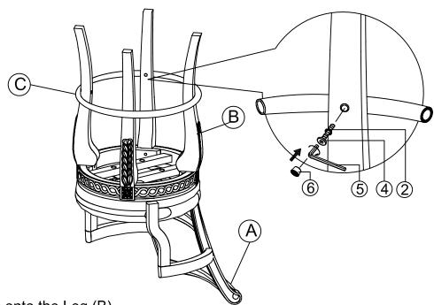
Put the Iron Hoop (C) onto the Leg (B). Insert the Lock Washer (2), Short Bolt (4) into each hole of the Legs (B) and tighten the bolt
