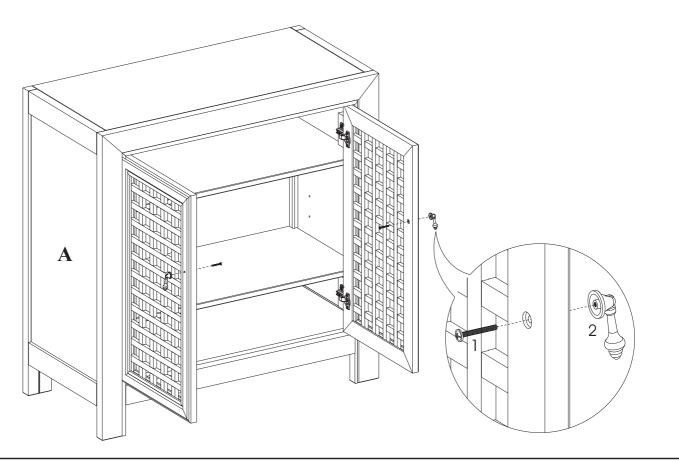
STEP 2: To adjust the shelves, loosen the screws of the support, lift the shelf and put the support at the wanted height and fix the screws again.
