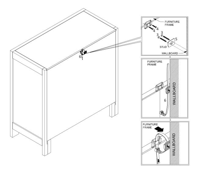
**STEP (A)** Locate a wall stud behind your furniture. Position a bracket on the stud approximately 1'' below the top of the furniture. Mark & drill pilot hole into the center of the stud with a 3/32" drill bit. Attach the bracket to the stud with the screws provided (3).
